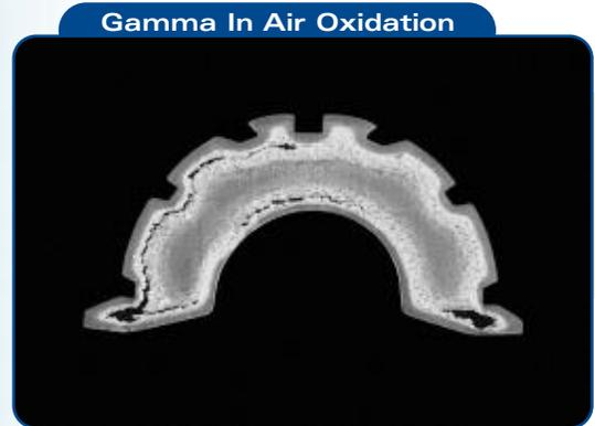
Shelf-aged, gamma in air-sterilized polyethylene demonstrating significant oxidation.
